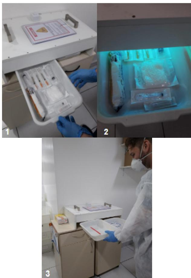
**Figure 1.** "UVC box" for disinfection of supplies returned to the pharmacy: portable device at different angles (1, 2 and 3) with two 18W lamps each.
